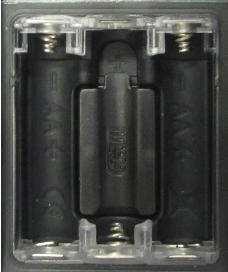
The polarity is clearly marked under each battery.
