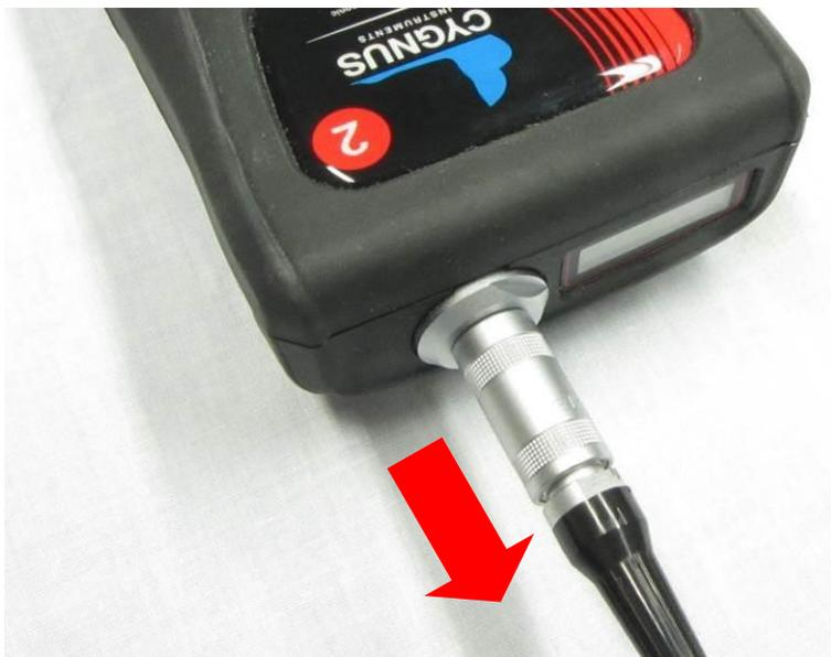
To release the connector simply pull back on the connector body. DO NOT pull the cable.
