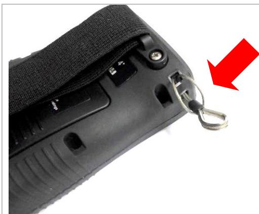
Wire loop fitted to the gauge body.
