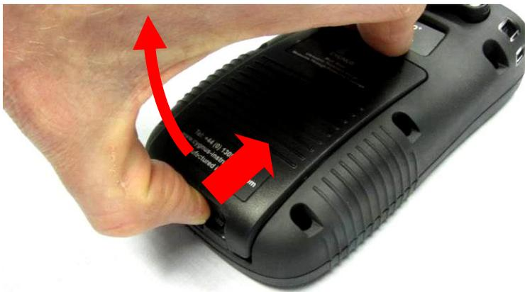
Press the bottom of the battery cover to release the retaining clip and lift up the battery cover.
