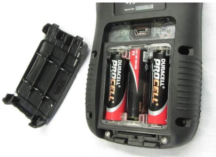
The batteries are located underneath.
