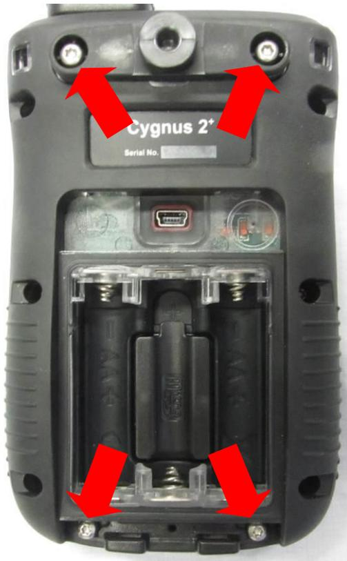
There are four Pozidrive screws holding the hand strap or Krusell® belt clip attachment in place. Two are under the battery cover.
