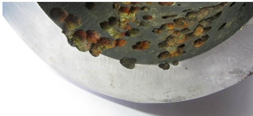
Large Corrosion Pits.
