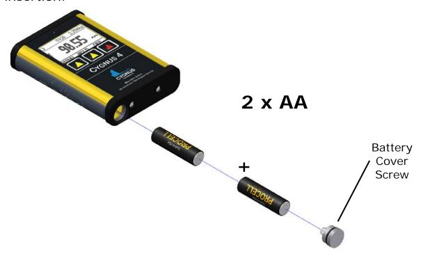
The Gauge can be fitted with NiCad or NiMH rechargeable batteries but this may reduce the specified operating time.
