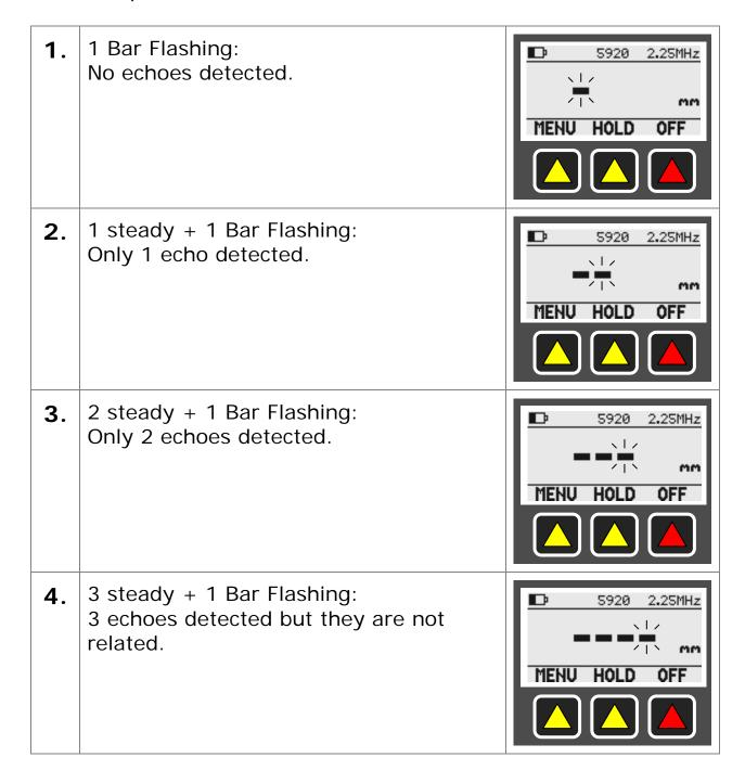
To help obtain a multiple echo reading the operator should continue to move the probe around to locate a suitable reflector, using a slight rocking motion.
