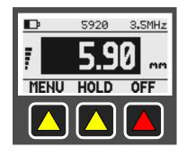
The gauge will alert the operator with a double 'beep' and also display the thickness value in a black box.
