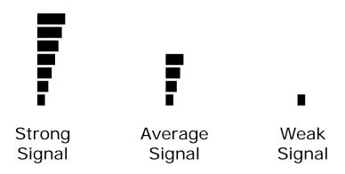
This coupling strength indicator shows a weak signal is being received.
