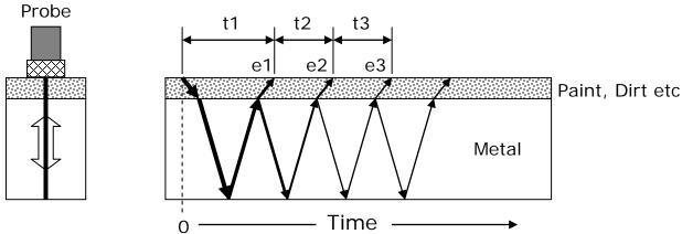
The *multiple-echo* beam travel is depicted above, spread out in time, to illustrate the timing method. In reality the beam path is straight and perpendicular to the surface as the ultrasonic energy reverberates up and down within the metal (shown on the left). Each time an echo is reflected back down, a small portion of the energy comes up through the coatings and is detected by the Probe which acts as a receiver (e1, e2 and e3).
