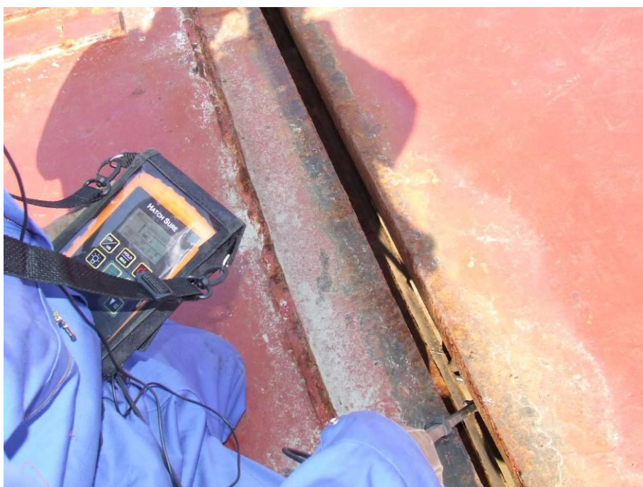
Fig 7.8. Scanning a Deep Hinged Joint.
