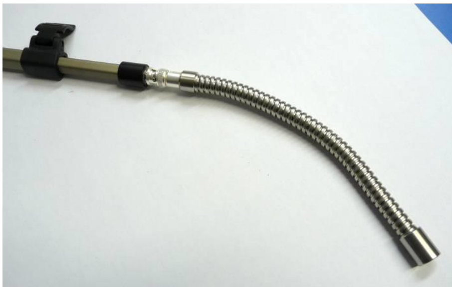
Fig 5.2 Inspection Microphone Connected to the Telescopic Extension
