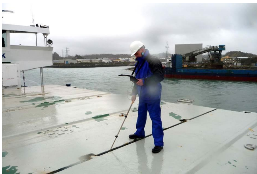
Fig 7.6. Scanning a Hatch Cover Joint.
