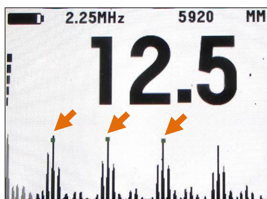
Flat, new steel 12.5mm thick.
