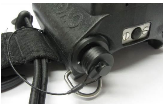
Probe Socket Cap Correctly Fitted.
