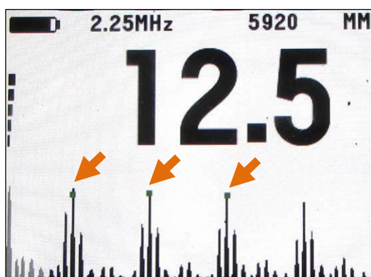
Flat, new steel 12.5mm thick.
