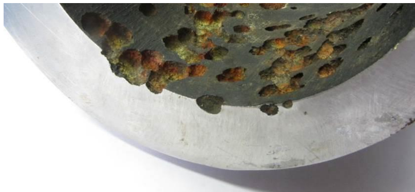
Large Corrosion Pits.
