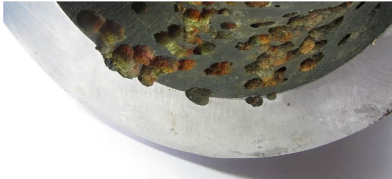
Large Corrosion Pits.
