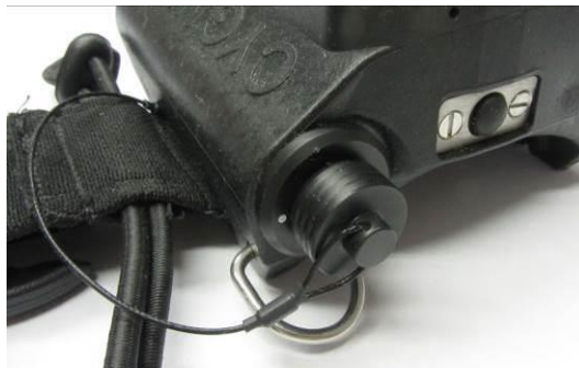
Probe Socket Cap Correctly Fitted.
