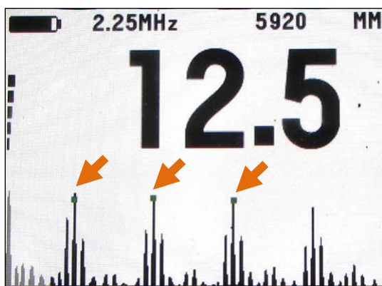
Flat, new steel 12.5mm thick.
