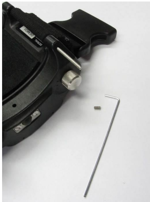
Wrist Strap Pin Securing Grub Screw
